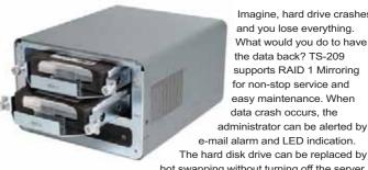
Imagine, hard drive crashes and you lose everything. What would you do to have the data back? TS-209 supports RAID 1 Mirroring for non-stop service and easy maintenance. When data crash occurs, the administrator can be alerted by e-mail alarm and LED indication.
